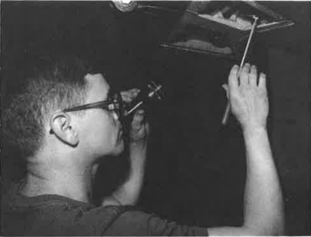
Technical Sgt. Ryland Y. Bailey used an inspection mirror to locate a foreign object in the aircraft wing assembly.
