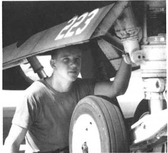
Sgt. Chuck Davis performs a nose-wheel inspection on one of the unit's A-7D Corsair II aircraft during the September UTA.
